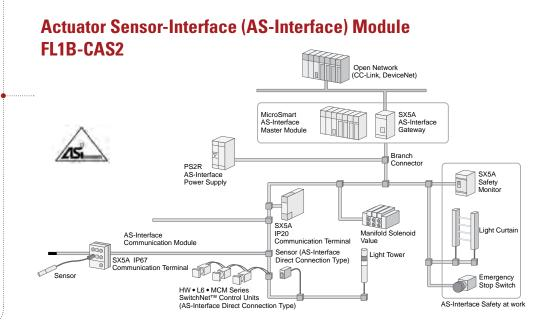
Primarily for control of sensors and actuators at distances of up to 100 meters, this interface utilizes the simplest and most-effective programmable control based industrial networking protocols, used in automation systems worldwide. Reducing the amount of engineering by employing simpler wiring, this module also enhances your operations by requiring little to no maintenance.
