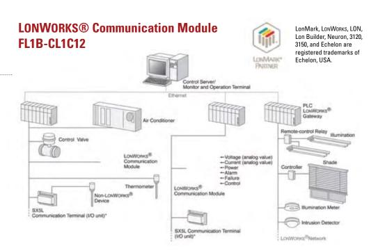
This communication module is an interface for connecting your IDEC SmartRelay to a Local Operating Network (LON). The LonWorks® communication module is a bus station on the LON and allows the IDEC SmartRelay to communicate with other LON devices.
