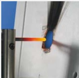
Burning behaviour: Glow wire test according to IEC 60 695-2-1: 750 °C, flame-retardant, self-extinguishing
