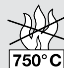
Burning behaviour: Glow wire test according to IEC 60 695-2-1: 750 °C, flame-retardant, self-extinguishing
