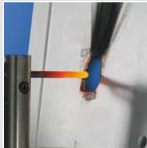
Burning behaviour: Glow wire test according to IEC 60 695-2-1: 750 °C, flame-retardant,
