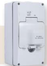
W66 (1000V / Leg) - DC21B up to 32A - 4 x M25 entries - Padlockable handle - Degree of protection IP66
