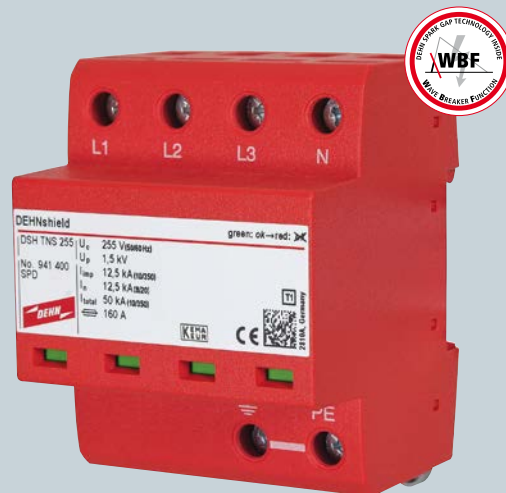
DEHNshield TNS DSH TNS 255 Part No. 941 400
