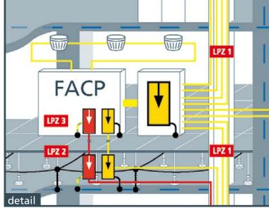
lightning equipotential bonding lightning current arrester / combined arrester
