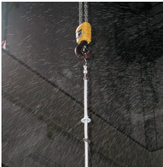
Figure 5.7.1.3 Withstand voltage test under wet conditions
