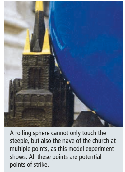
Figure 5.1.1.2 Model of a rolling sphere; source: Prof. Dr. A. Kern, Aachen
