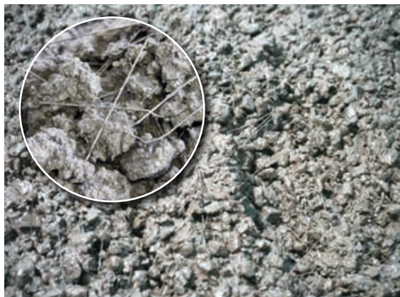
Figure 5.5.2.27 Fresh concrete with steel fibres
