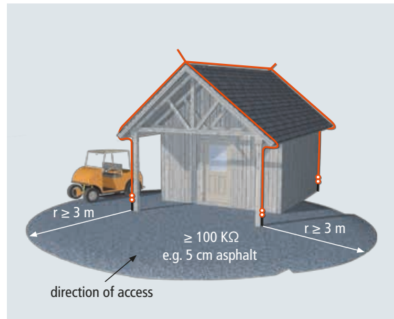
Figure 9.23.1 Protection of a shelter with one entrance and defined direction of access against step and touch voltage
