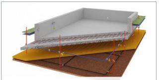
Ring earth electrode Foundation with increased earth contact resistance Ring earth electrode with functional bonding conductor according to DIN 18014
